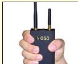
These devices will disrupt the local cell phone signals by preventing the phone from using the control channels to communicate with the cell tower. Using this device will generate .6 watts of power (using 2 antennas). It should disrupt all signals within about 10 meters. However, this may not work because some cell
